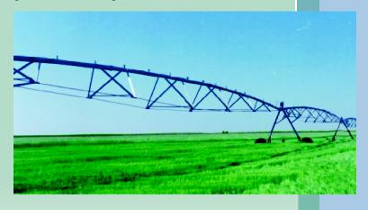
The span structure is coated with special resistant to high salty water paint that has proven itself durable in marine equipment. Galvanized structure is also available upon request.
